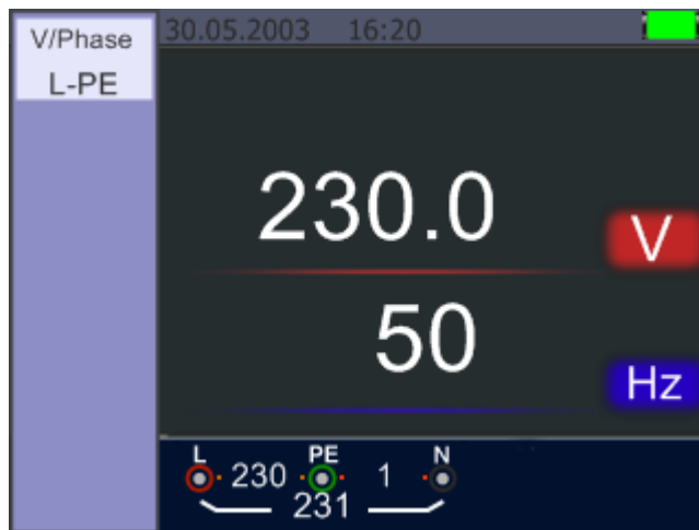
Figure 20 Screen while measuring Voltage and Frequency
