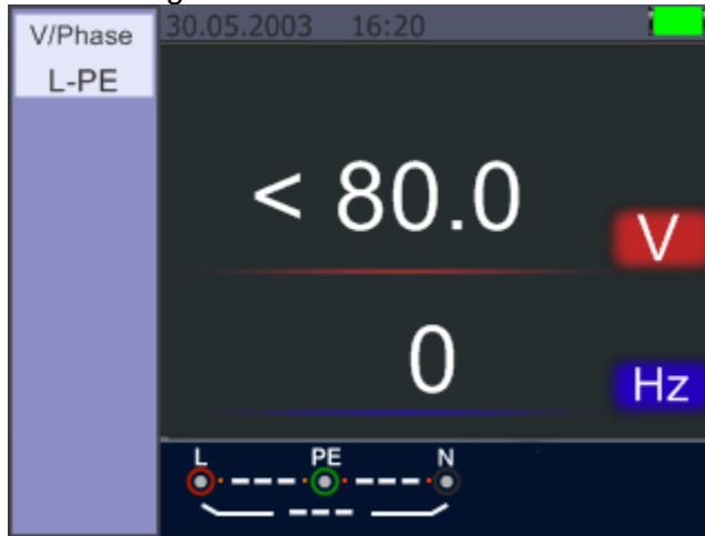
Figure 19. Standby screen for the Voltage and Frequency
