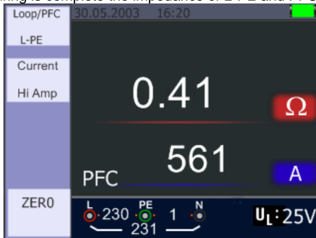
Figure 9 Hi Amp LOOP – Measurement finished
