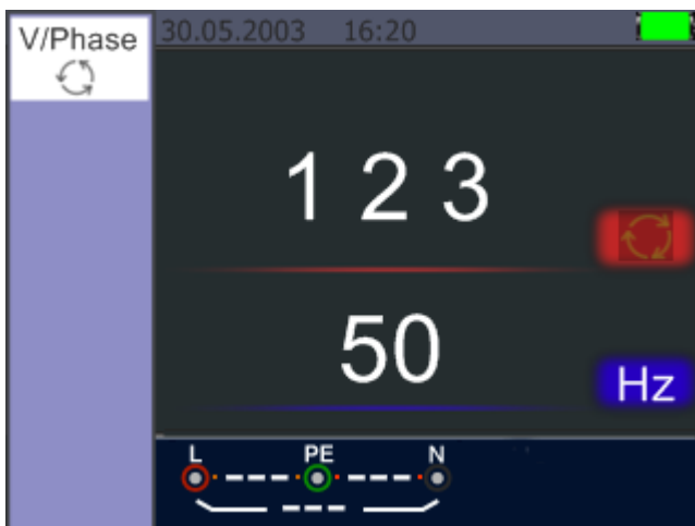
Figure 23 Phase Sequence screen -when connected in clockwise direction.
